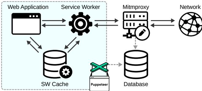
Figure 2: Automation framework to record accesses to the Service Worker Cache.
