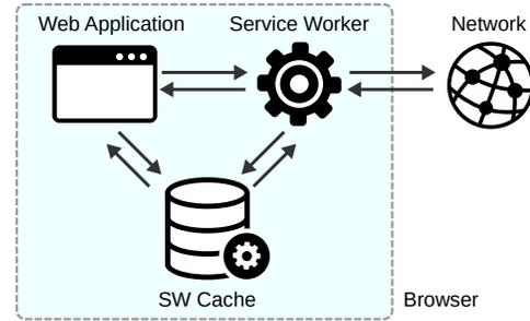
Figure 1: Service workers sit between web applications and web servers. They can store HTTP content in the cache and serve them to web pages, e.g., to speedup the navigation.
