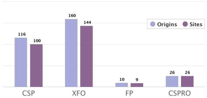
Figure 3: Security policies found on cached HTML content. These policies can be bypassed by altering cached responses, thereby voiding their effects on the security of the page. The most widespread policies include Content-Security-Policy (CSP), X-Frame-Options (XFO), Feature-Policy (FP) and Content-Security-Policy-Report-Only (CSPRO).
